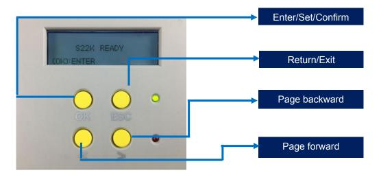
Step 3: LCM show "Clean function" press "OK" one time. Then LCM will show "Open the cover".
