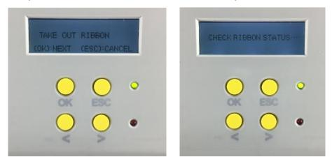
Step 6: The cleaning card will be exit from card exit mouth after finished cleaning. After it, please install the ribbon cartridge and close the upper cover.
