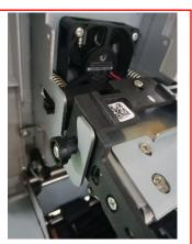
Find the wiring and pull it out from the wiring plug with your hand.
