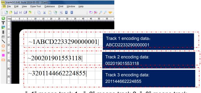
"~1" means track 1 , "~2" means track 2, "~3" means track 3. "|" means stop code.
