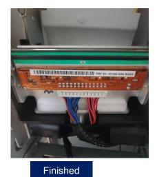
Clip the print head onto the hook and hold part A against part B until the cylinders on both sides of part A are stuck on the metal hook.
