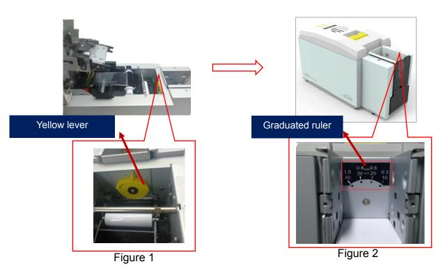
Figure 1: The feed card thickness needs to be adjusted according to the card's actual thickness
