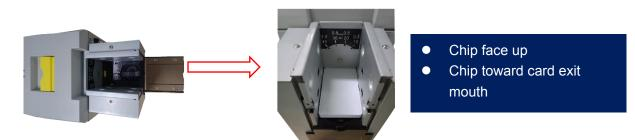
Contact chip cards require the chip face up, otherwise data can not be read or written to the chip card. (Put the card like an ATM direction)
