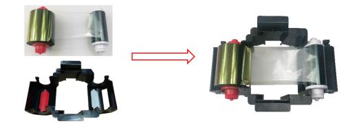
Red roller supply with unused ribbon. White roller supply with used ribbon.
