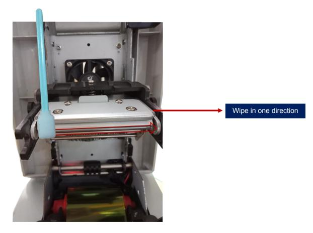
Avoid print head direct contact with metal objects, sharp objects or fingers, and do not contaminate any liquid to clean the print head.
