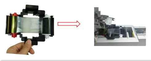
Ribbon mounting direction: Red roller close to the Back-end card exit mouth(left), white roller close to the input hopper (right).
