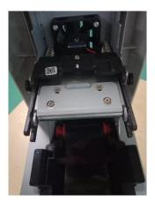
Step 6: Enter the new print head serial number into the driver. Failure to enter may result in an abnormal print.
