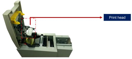
Step 3: Look closely at the mounting structure on both sides of the print head.
