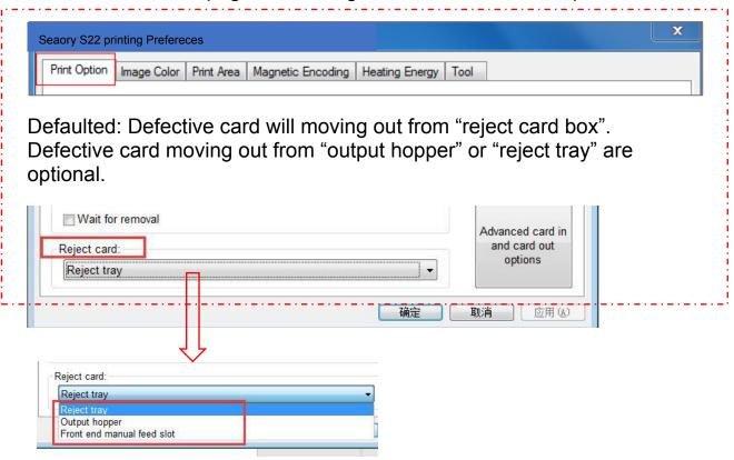
Generally reject card box will be used when reading and writing chip cards.
