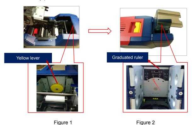
Figure 1: The feed card thickness needs to be adjusted according to the card's actual thickness
