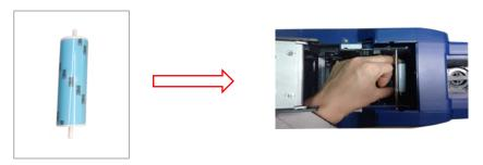
The purpose of cleaning roller is to absorb the dust on the card and card feeding roller, improve the printing effect.
