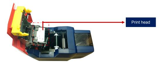
Step 3: Look closely at the mounting structure on both sides of the print head.
