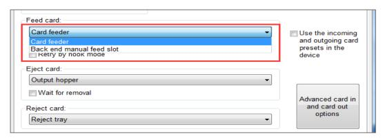
(2) Manual feeding card piece by piece from back end manual feed slot is optional.
