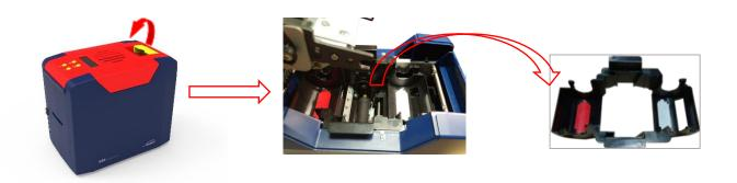
Step3: In order not to interupt the normal work of card printer, please follow below image to take out of the pearl wool which inside the printer(It's unneccessary to place pearl wool when card printer is normal working)
