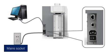
Ethernet communication interface installation: RJ45 network interface ,568B connection mode.
