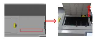
(3) Install the assembled cleaning module above (press vertically) into the card printer as shown in the picture below:
