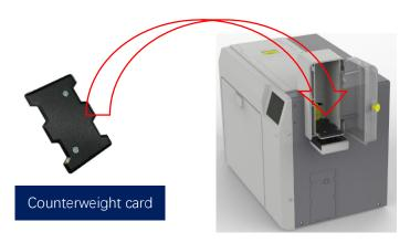
Counterweight card: Apply gravity to the card to ensure stable card insertion when the number of cards in the card slot is small.
