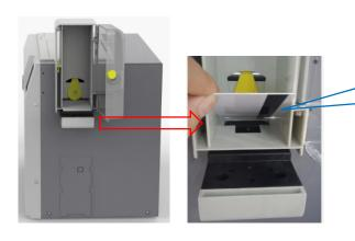
As shown in the figure, the magnetic stripe is facing the lower right.
