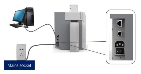
Ethernet communication interface installation: RJ45 network interface ,568B connection mode.
